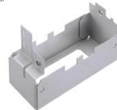
Alternatives to welding: flanges can be bent and side elements can be secured in place using pins that fit into holes.
