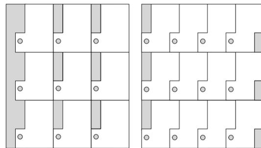
Using design to reduce scrap: designing parts so that they nest closer to one another is a way to maximize sheet utilization.
